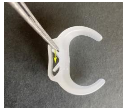
Figure 8. Use of forceps to tighten expansion flaps.
